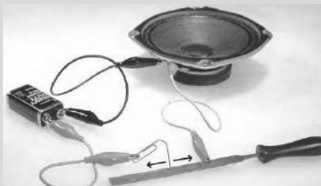
Figure 5.2 Scratching a speaker.
