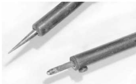
Figure 6.1 A happy soldering iron (top) and a sad soldering iron (bottom).
