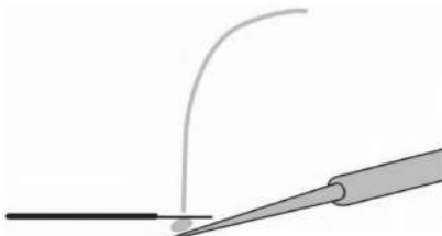
Figure 6.2 Tinning a wire.
